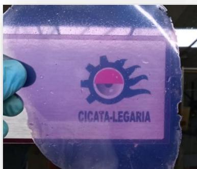
**Figure 1.-** CoDMCM membrane from the casting method
